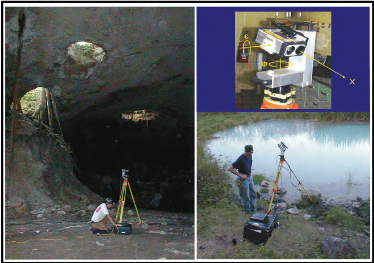
Figure 3.6. LIDAR SCANNING OF CENOTE SURFACE FEATURES. Top image shows the Riegl LPM98-VHS Lidar scanner with the two instrument rotation axes and distance measurement. \epsilon - tilt axis (degrees); \phi - pan axis (degrees); x – range value (meters). Two Lidar scanning sites are shown. On the left, the large cave of Caverna Cuarteles are imaged. The right hand photo shows scanning of the cenote of Azufrosa. (Photographs by Bill Stone and Marcus Gary.)
