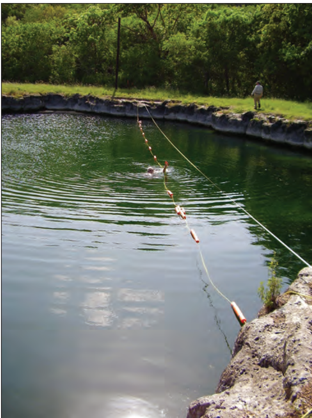
Figure 4.3. ERI ELECTRODES ACROSS LA PILITA WATER SURFACE. Photograph shows placement of electrodes across the water surface of La Pilita. These data were used to check the electrical method's ability to locate water-filled voids.
