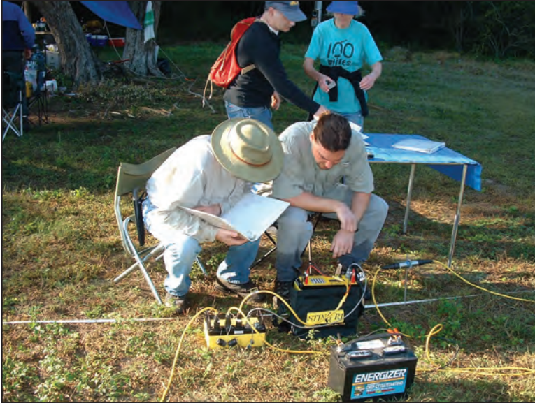
Figure 4.2. AGI STING ELECTRICAL RESISTIVITY CONTROL UNIT. Photograph shows operation of the AGI sting R1 electrical resistivity instrument at La Pilita in 2003 (photograph by Robin Gary).
