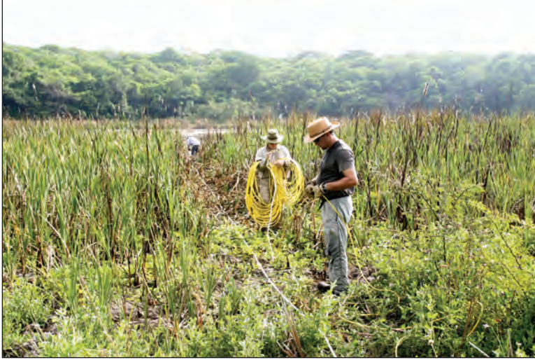
Figure 4.5. ERI TRANSECT LINE IN TULE. A significant drought in 2006 dried up the water in Tule, making geophysical surveys logistically feasible. Above photo shows installation of the ERI transect from the southwest end of the line (photograph by Jim Bowden).
