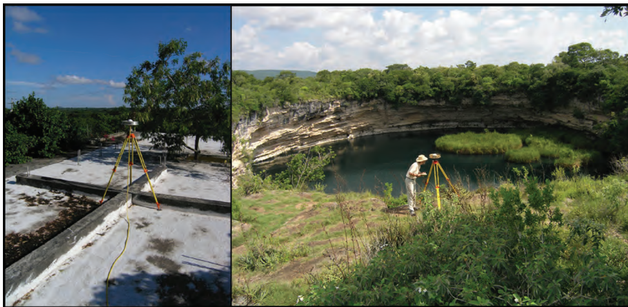
Figure 3.4. CARRIER PHASE DIFFERENTIAL GPS SURVEY INSTRUMENTS. Photographs show the Trimble 4000 SSI GPS receivers used to georeference benchmarks that register lidar, sonar, and water level data in true geographic coordinates. The photo on the left shows the base station set up on the roof of the ranch house to collect position data continuously over the 5 day survey period. The photo on the right shows set up of the “rover” unit at a benchmark on the south rim of El Zacatón.
