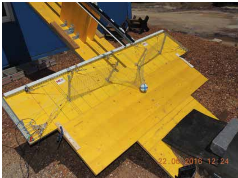
Fig. 2: arrangement for lab-scale testing (vertical 90° vs inclined 30°)
