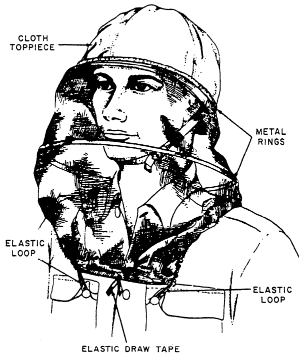
Figure 2-36.—Mosquito hat and net over helmet.
