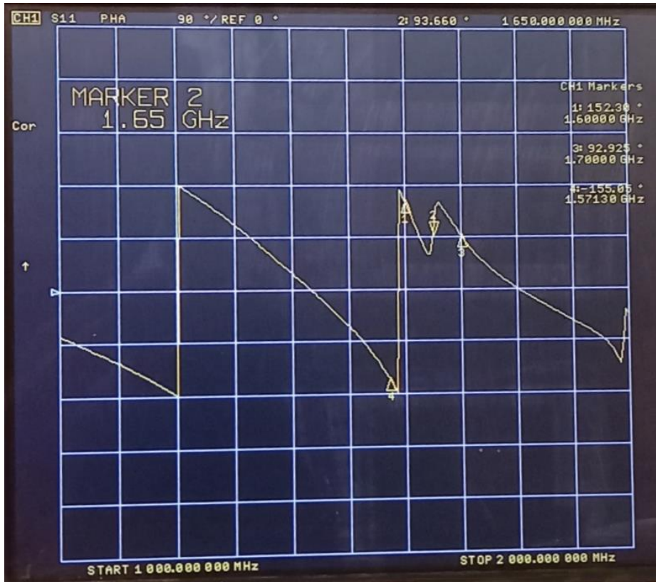
S11 Phase: one can see that phase change has a positive slope around 1650 MHz +/- a few MHz. This is the result of two resonances slightly above and below the center frequency.
